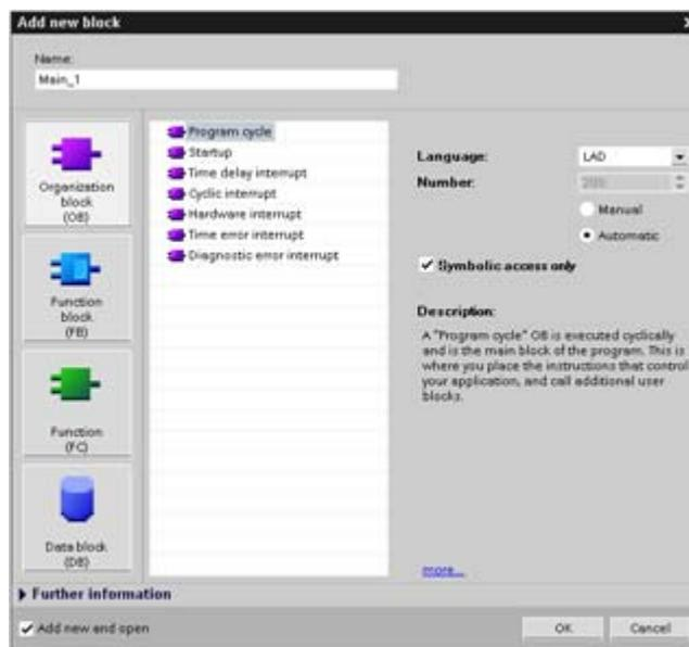
You can create other OBs to perform specific functions, such as startup tasks, for handling interrupts and errors, or for executing specific program code at specific time intervals.
