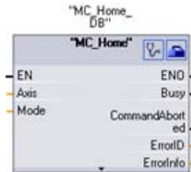
MC\_Home establishes the relationship between the axis control program and the axis mechanical positioning system.
