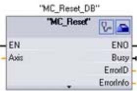
MC\_Reset resets all motion control errors. All motion control errors that can be acknowledged are acknowledged.
