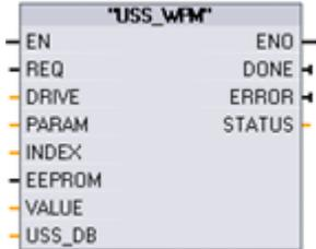
The USS\_WPM instruction modifies a parameter in the drive. Execute the USS\_WPM from the program cycle OB. Minimize the number of EEPROM write operations to extend the EEPROM life. Use the "EEPROM" parameter to disable writing to the EEPROM.
