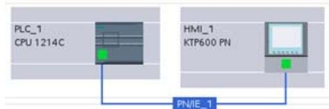
A network connection is created for the two devices.
