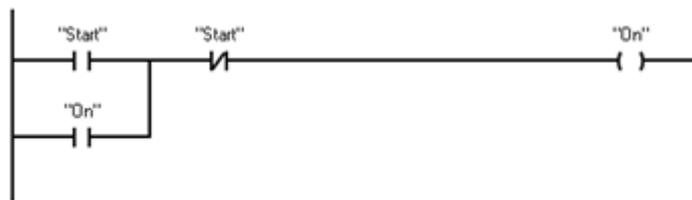
The elements of a circuit diagram (such as normally closed contacts, normally open contacts, and coils) are linked to form networks.
