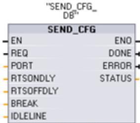
The dynamic configuration changes are not permanently stored in the CPU. After a power cycle, the initial static configuration from the device configuration will be used.
