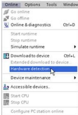
If you are connected to a CPU, you can upload the configuration of that CPU, including any modules, to your project. Simply create a new project and select the "unspecified CPU" instead of selecting a specific CPU. (You can also skip the device configuration entirely by selecting the "Create a PLC program" from the "First steps". STEP 7 Basic then automatically creates an unspecified CPU.)
