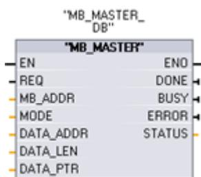
The MB\_MASTER instruction allows your user program to communicate as a Modbus master. You can access data in one or more Modbus slave devices.
