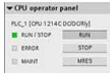
Use the button on the operator panel to change the operating mode (STOP or RUN). The CPU panel also provides an MRES button for resetting the memory.
