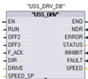
The USS\_DRV instruction exchanges data with the drive, by creating request messages and interpreting the drive response messages. All of the USS instructions associated with one USS network and CM must use the same instance DB.
