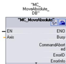
MC\_MoveAbsolute starts motion to an absolute position. The job ends when the target position is reached.
