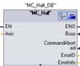
MC\_Halt cancels all motion processes and causes the axis motion to stop. The stop position is not defined.
