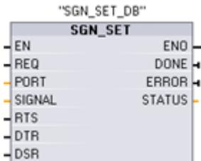
The SGN\_SET and SGN\_GET are valid only for the RS232 CM module. Use these instructions to read or set the RS232 communication signals.
