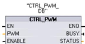
When placing a CTRL\_PWM instruction into the program editor, a DB will be assigned. A data block (DB) is used by the CTRL\_PWM instruction to store parameter information. The data block parameters are controlled by the CTRL\_PWM instruction.
