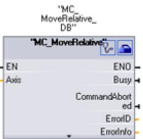
MC\_MoveRelative starts a positioning motion relative to the start position.
