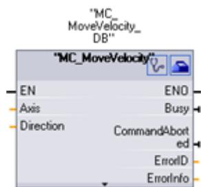
MC\_MoveVelocity causes the axis to travel with the specified speed.
