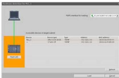
After you select the CPU from the online dialog, STEP 7 Basic uploads the hardware configuration from the CPU, including any modules (SM, SB, or CM).
